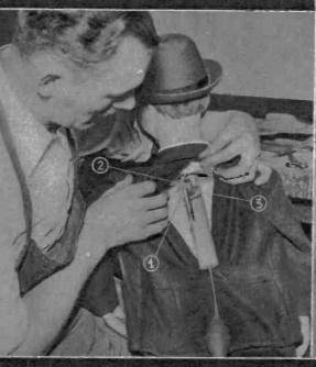
16 Lever (No. 1) and the bulb control the mouth movements, cord (No. 2) works the winking eye, ball (No. 3) rolling eyes
