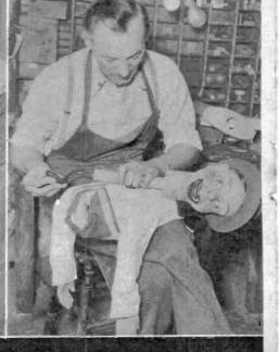
15 The mouth movement is a beliews made of innertube patches, controlled by a bulb
